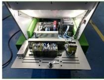
Electrical cabinet inside the machine for better protection and better adaption to working space.
