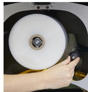
Movement of the ring to position the reel holder is done by hand by moving the ring from the outside protective yellow cover
