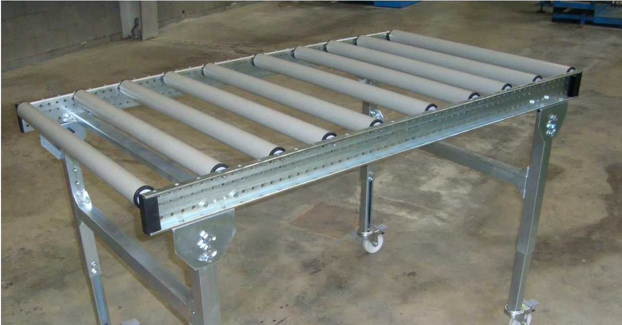
Example of gravity pvc roller conveyor (casters not quoted, optional) Usually the same length at the infeed and outfeed side, to cover the total of the maximum product length. Support until 50 Kg / linear meter – Gap between rollers: 150 mm – Diameter of PVC rollers: 50 mm
