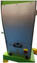
Electrical cabinet inside the machine for better protection and better adaption to working space.
