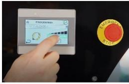
Touch screen and Emergency button at the front of the machine for better accessibility.
