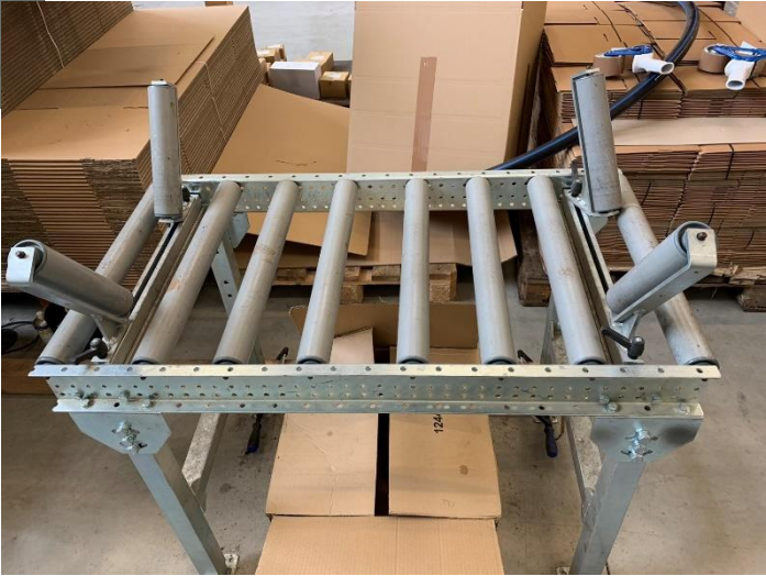
Example of “V shape” vertical rollers on a gravity pvc roller conveyor. For round products or bundle of tubes, etc.. that have to be hold before wrapping. Vertical rollers can move towards the center of the conveyor sliding by a guide. Distance between vertical rollers should be informed before manufacturing because the guides are welded to the conveyor structure.
