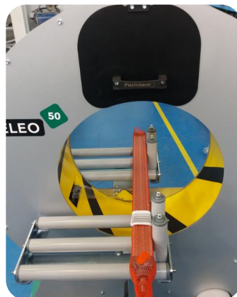
Small table with vertical rollers can be positioned up & down – left & right. Adapted to your wrapping needs depending on the product you have.
