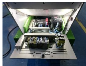
Electrical cabinet integrated inside the machine for easy fitting in any packaging space.
